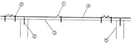
1. **Metal Roof Deck Panels\*** — No. 29 MSG min thick coated steel. 24 in. cover width (26 in. overall width). **BENTON METAL DEPOT INC** (<u>View Classification</u>) — "5V Panel"
